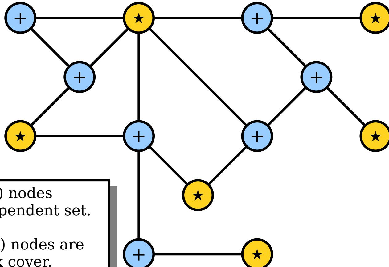
**Theorem:** Let  $G = (V, E)$  be a graph and let  $C \subseteq V$  be a set. Then  $C$  is a vertex cover of  $G$  if and only if  $V - C$  is an independent set in  $G$ .
